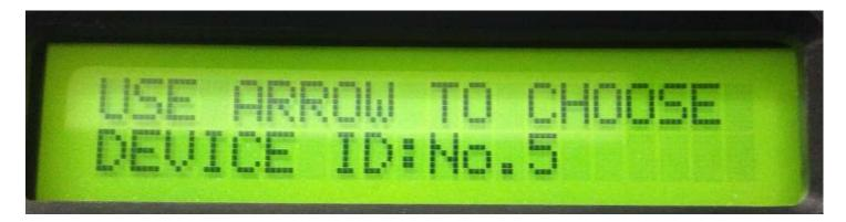
After pressing "Enter" key, the door of the cabinet will open, and the admin can place the device into the cabinet.
