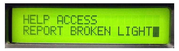
Press "Enter" button on the keypad, type in the port number and the broken light is added into the database.
