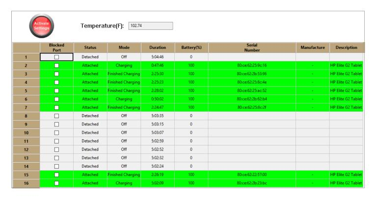
When we want to block a port, we can select "Blocked Port" column of the related line, and press "Save Changes" button, the information will be saved to database.
