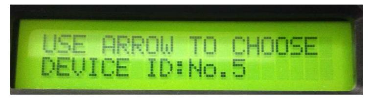
When having found the device you want to remove, press "<u>ENTER</u>" button, and the item will be removed from the checkout list of the database.
