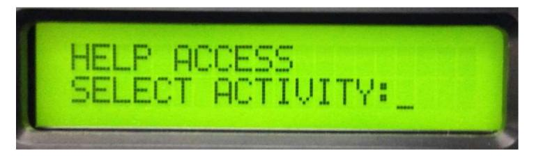
Scroll the display with the arrow buttons on keypad, until the following screen is shown:
