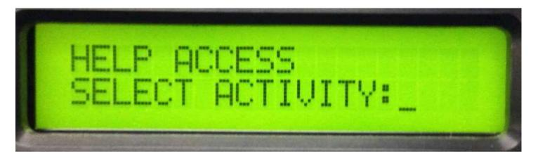
Use up and down arrow on the keypad to choose the options, until see "Report Broken Device", press return button to choose, and then follow the standard procedure to check in. It does not matter the device is plugged in or not.
