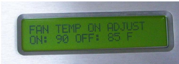
*Illustration 32: Mode to Adjust the ON Temperature of the Fans.*
