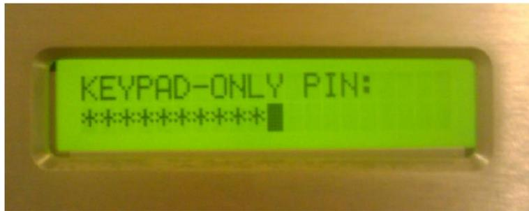
*Illustration 5: LCD Display for PIN Keypad Entry after 10-digits*
