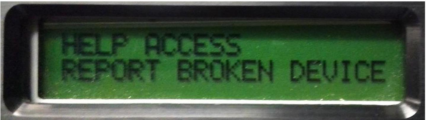
Scan the badge and place the device in the drawer when the drawer is open. The device will be added into the database as broken, and the device is also labelled as check-in.
