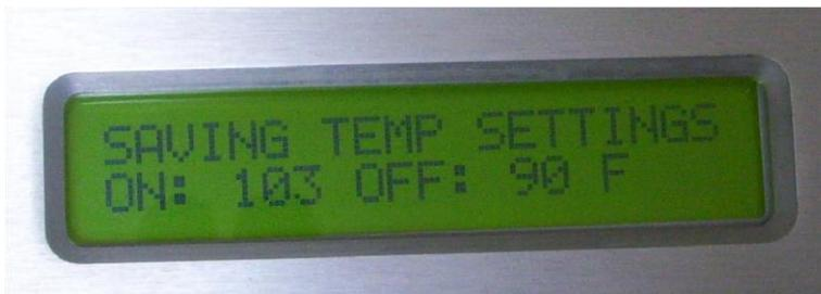
*Illustration 33: Saving the Temperature On/Off Settings of the Fans.*
