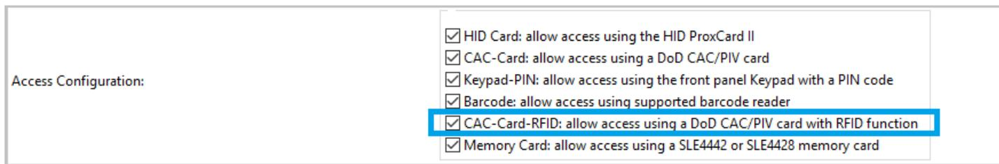
After CAC-Card-RFID is selected in Access Configuration, the user can use either CAC (with PIN) or RFID for the device checking in or checking out, and the management system will regard it as the activity of the same person. Basically, the user can use CAC function to check-in and checkout, or use CAC to check out and use
