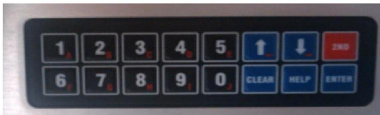
Illustration 4: Keypad. Used for PIN Entry and System Admin Functions.
