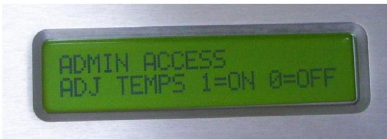
*Illustration 31: Adjust either the Turn-On Temperature, or Turn-Off Temperature of the Fans.*
