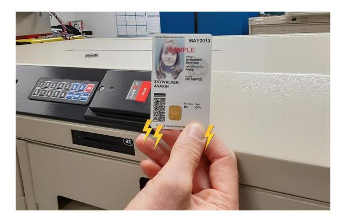
b) Place the card on the surface of the cabinet for a moment. The chip of the card needs to touch the cabinet, so that the electricity on the chip can be discharged.
