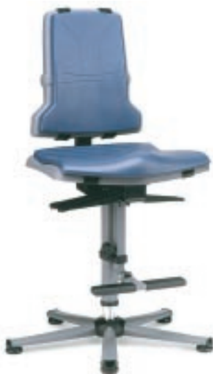
Model 9811 with contact backrest and seat tilt adjustment, mounting step, glides, and optional integral foam upholstery in blue. The mounting step moves when adjusting seat height and swiveling, and folds-up when not required.
